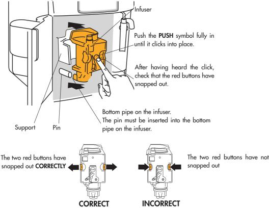
Check that the two red buttons have snapped out, otherwise the door cannot be closed.
